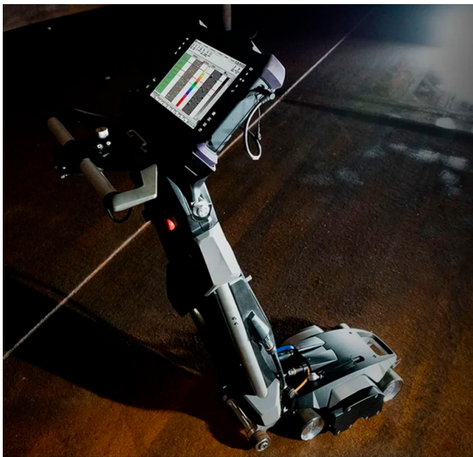
Figure 3: FloormapX MFL tank bottom inspection.
